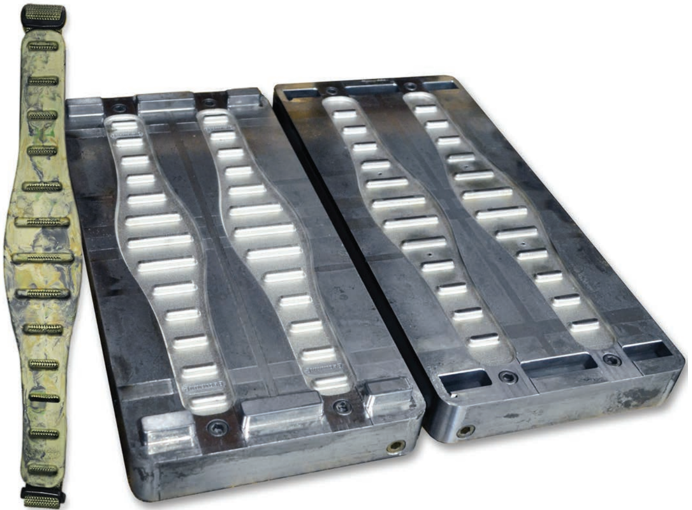
4.68 Two Halves of a Mold Used to Form a Strap (shown at left). (Two straps can be molded at once.)
