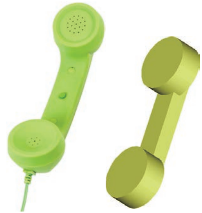
4.59 Complex Shapes. The 3D solid primitives in this illustration show basic shapes that make up a telephone handset. (Photo copyright Everything/Shutterstock.)
