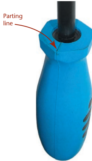
4.67 Parting Line. The parting line on a molded part is often visible as a ridge of material.
