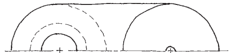
4.65 Orthographic sketches of symmetrical parts may show only half of the object.
