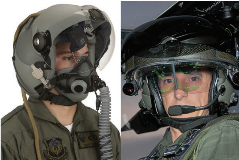
Figure 17.10 This image shows two head-mounted displays currently in use within U.S military aircraft. On the left is the GENTEX Scorpion Helmet-Mounted Cueing System in use within the A-10 Thunderbolt and the Air National Guard/Air Force Reserve F-16 Block 30/32 Viper aircraft. On the right is the Thales TopOwl Helmet-Mounted Sight and Display that is operational in five major helicopter programs across 16 countries, including the Cobra AH-1Z and Huey UH-1Y.
