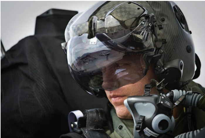
Figure 17.11 This image shows an oblique view of the F-35A Lightning II helmet-mounted display, which provides pilots unparalleled situational awareness, with real-time imagery from six sensor packages mounted around the exterior of the aircraft.
