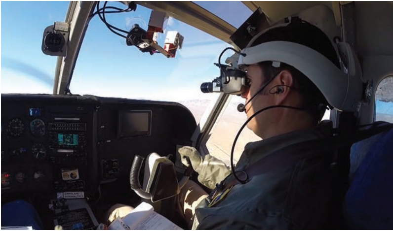
Figure 17.1 The Fused Reality head-mounted display shown in this image provides the user a combined view of the actual cockpit interior and instruments as well as computer-generated imagery beginning at the windows.
