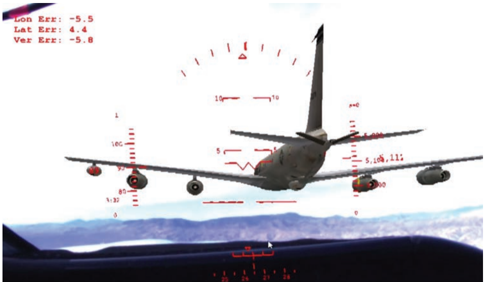
Figure 17.3 This image shows the Fused Reality system operating in stencil mode, within which a computer-generated virtual tanker is displayed over the real scene of the outside world.
