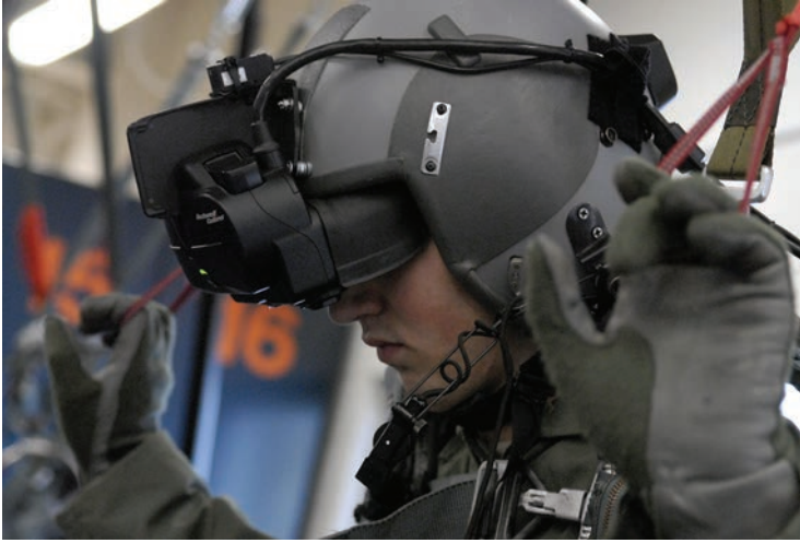
Figure 17.6 The PARASIM Virtual Reality Parachute Simulator includes a stereoscopic wide field of view (FOV) head-mounted display and sensors to track the orientation of the user's head.
