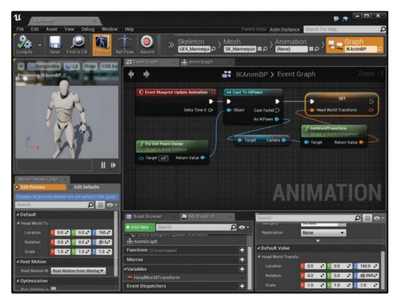
Figure 7.8 Animation Blueprint: head transform setup
