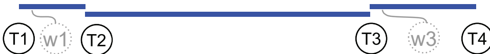
Figure 6.6 Diagram of one RPC, showing the four times. T1 to T2 is the time from client user-mode code sending an RPC request to server user-mode code receiving that request. T2 to T3 is the server time spent performing the request. T3 to T4 is the time from server user-mode code sending the RPC response to client user-mode code receiving that response. Times T1 and T4 are taken from the client CPU’s time-of-day clock, while T2 and T3 are from the server CPU’s time-of-day clock. The two clocks may be offset from each other by microseconds to milliseconds. We will deal with clock alignment in the next chapter. w1 is the time the client kernel-mode code sends the request to the network hardware (“w” for “wire”), and w3 is the time the server kernel-mode code sends the response to the network hardware.
