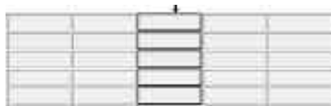
Figure 10.27 When you mouse over the top table border, the mouse pointer turns into an arrow that you can click to select a column. Use the left table border to select a row.
