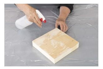
**FIGURE B.3** Wetting the wood raises the grain for sanding so it won't raise again later.
