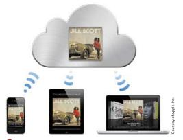
Apple's graphical depiction of iCloud. Changes made on one device are pushed to the cloud (a remote data center) and then synced automatically with your other devices.
